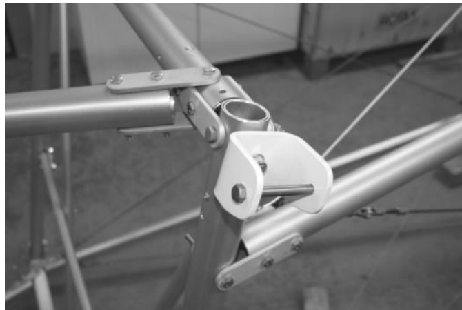
Figure 22 Port end of the upper rear cabin cross-piece.
