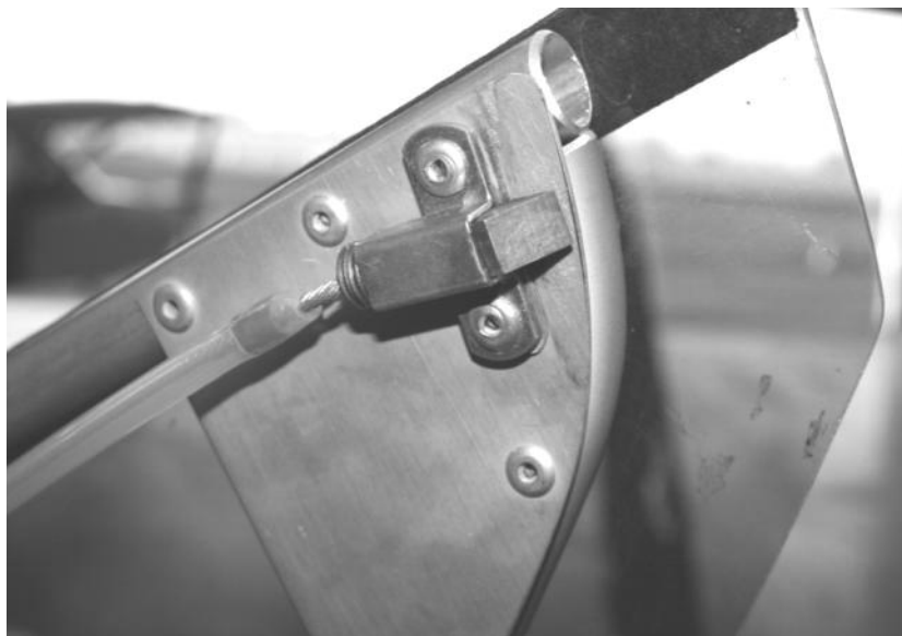
Figure 312 rear gusset plate and rear end of lower door.
