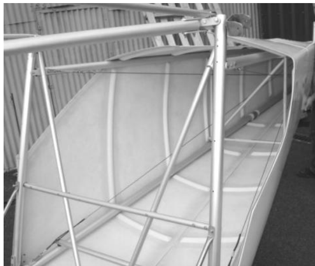
Figure 117 fitting the rear fairings in position.
