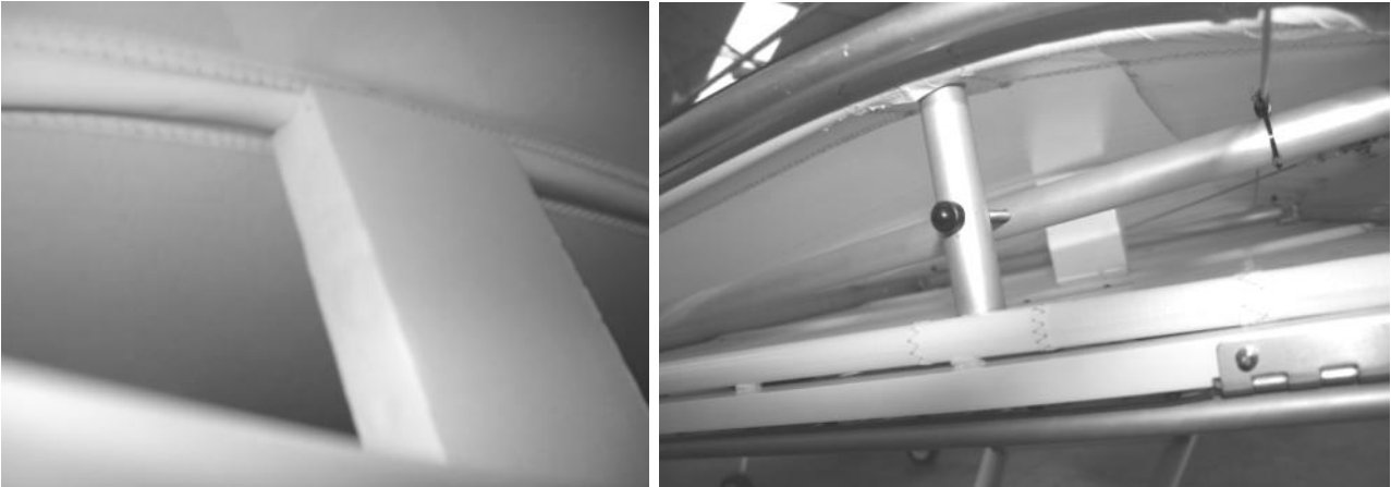
Figure 358 wing profile support blocks
