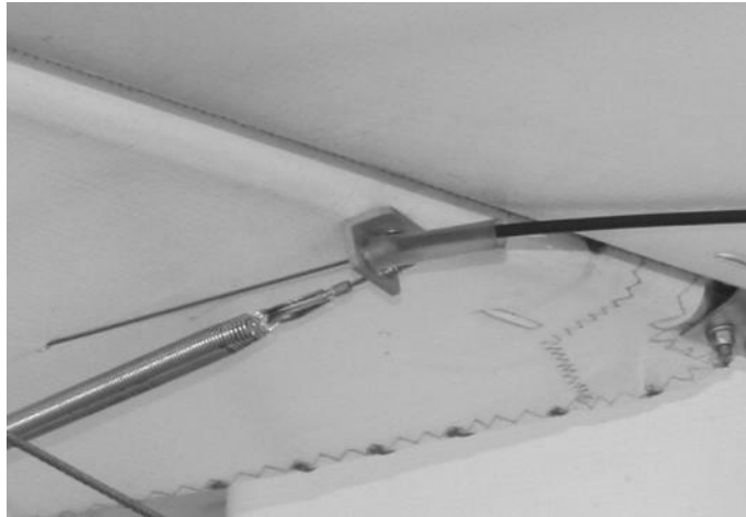
Figure 317 aft end of trimmer cable.
