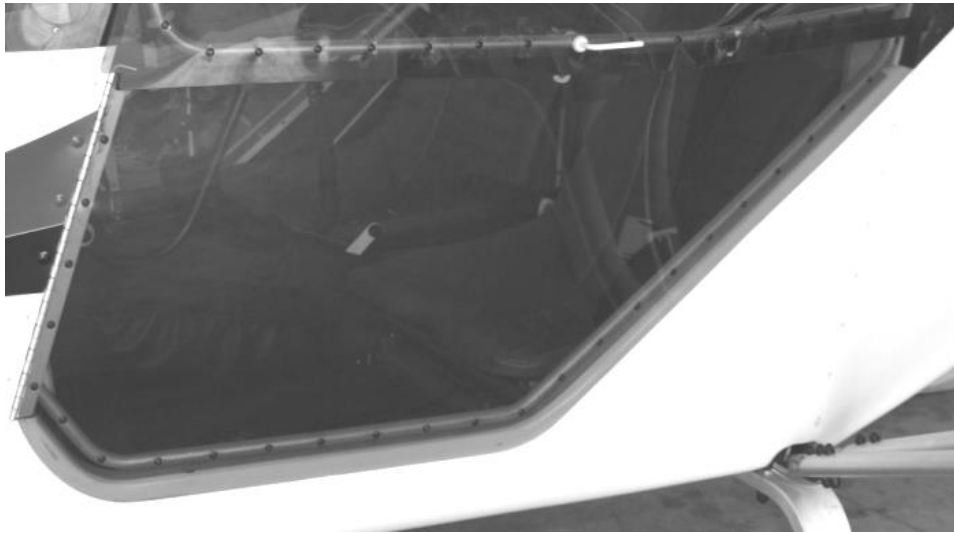
Figure 318 lower door lexan fit
