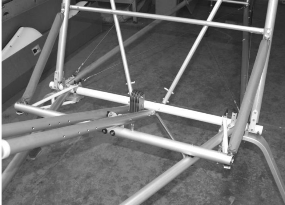
Figure 16 Tu9 (The big white tube), looking from above, front of aircraft to left
