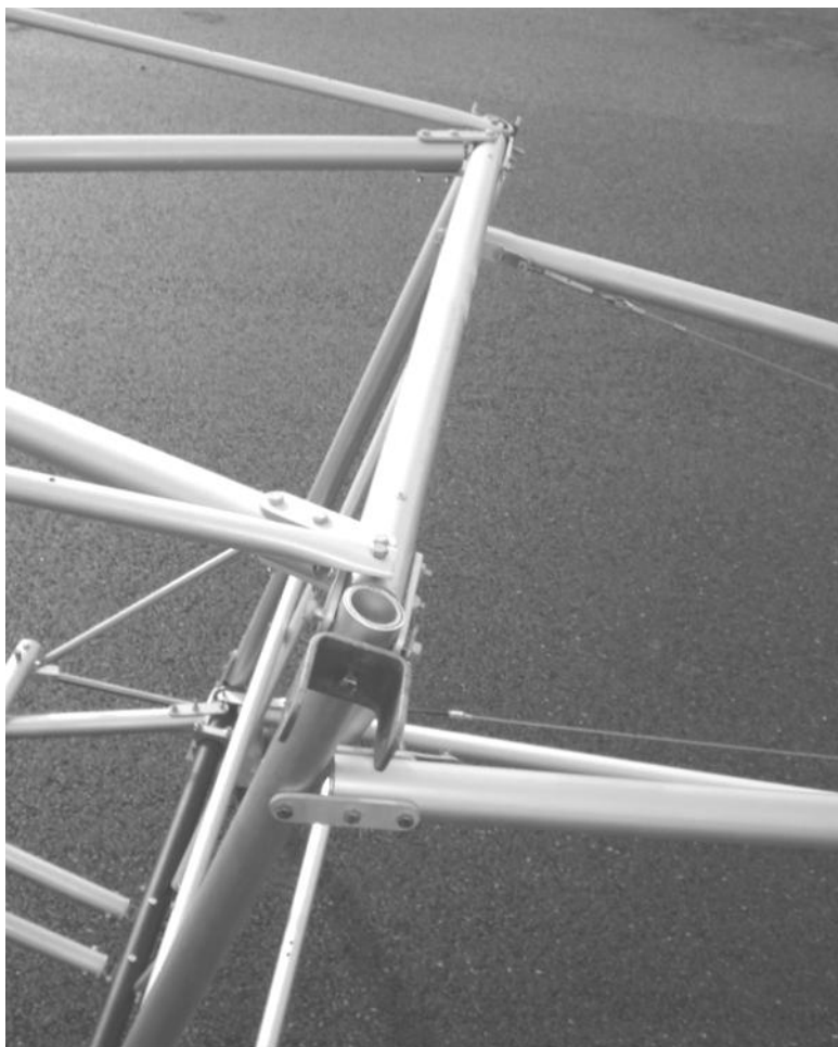
Figure 14 Cabin upper rear corner
