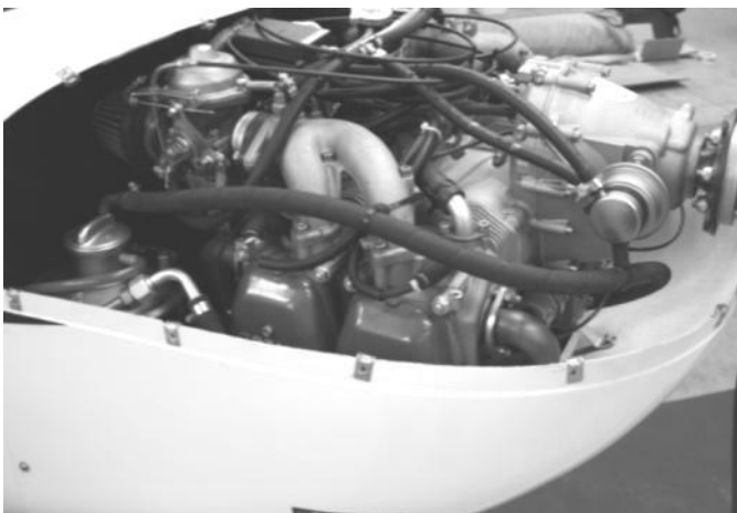
Figure 205 routing of oil hose from oil cooler connection to outlet on oil tank. Note use of cableties through short lengths of fuel tubing to act as standoffs on fuel pump and inlet manifold to secure hose.
