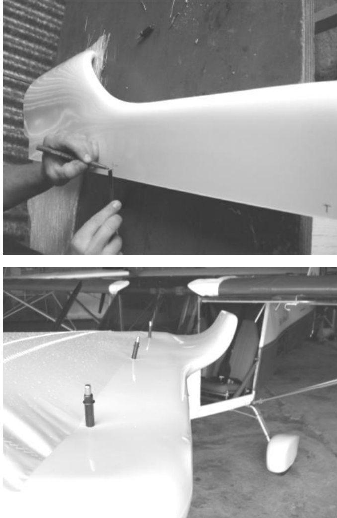
Figure 357 marking, drilling and fixing the wingtip fairings.
