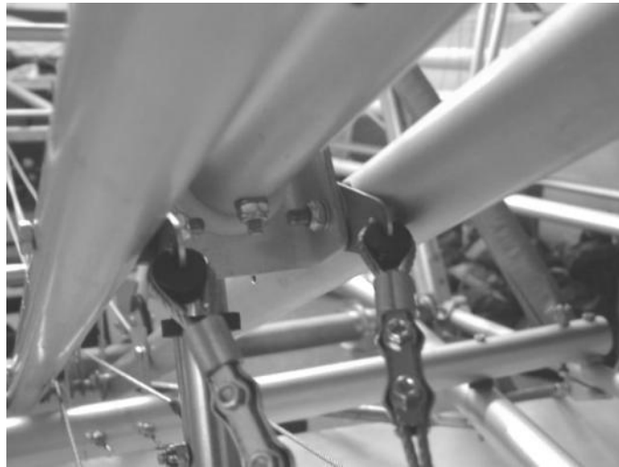
Figure 114 rudder stop cable adjustment.
