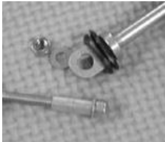
Figure 369 Upper fixing hardware. Note position of rubber grommet (bolt may be superseded with 6mm bolt)
