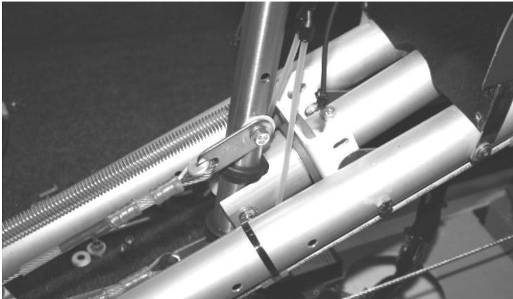
Figure 108 Nynja elevator cable connection on control stick. (Note: hole closest to pivot used, and that a thin plastic washer is fitted between tang and stick)
