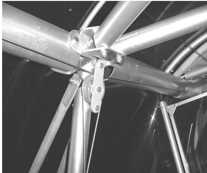
Figure 150 aileron cable fuselage pulleys.
