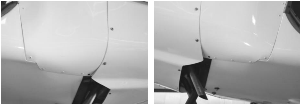
Figure 196 fixing lower edges of Scuttle moulding
