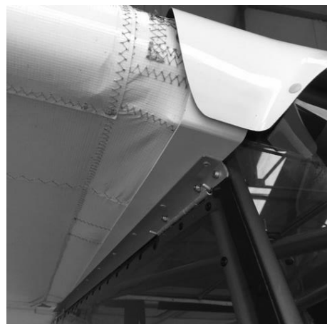
Figure 297 fabric enclosure, and extended angle to close gap to wing undersurface rivetted to top of angle.
