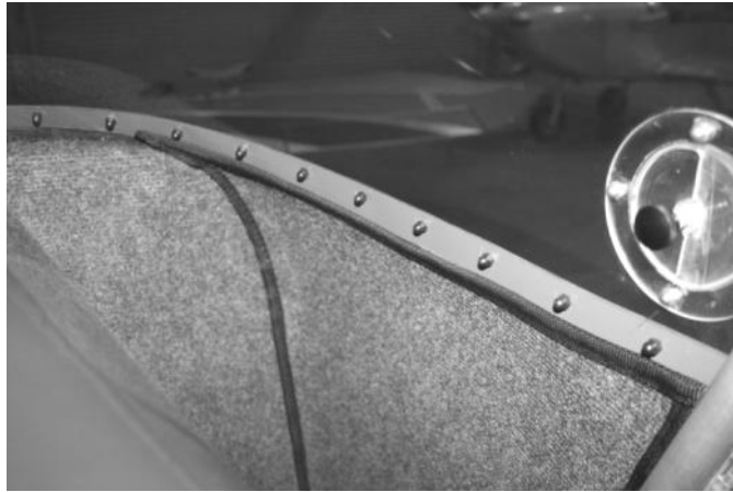
Figure 291 windscreen over lap inside cowling (note we painted the overlap to match interior fabric trimming.
