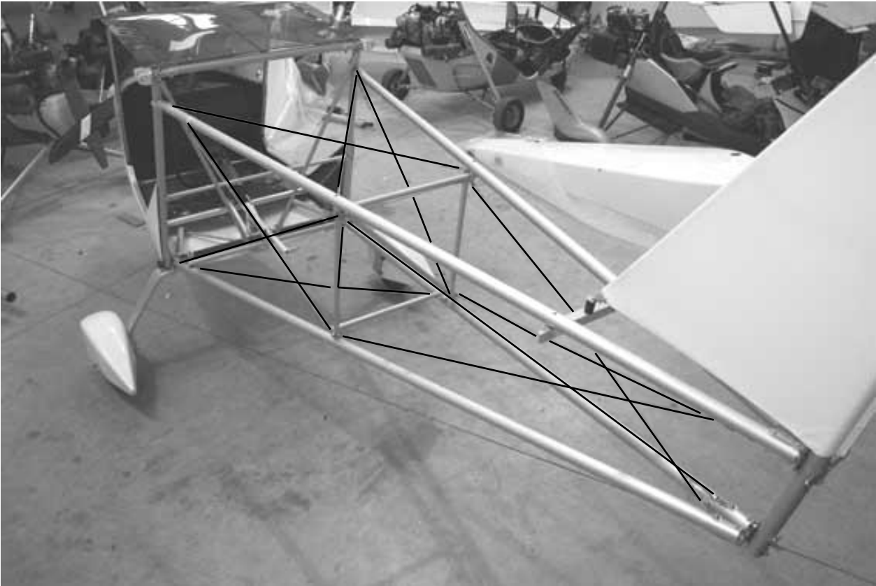
Figures 65 cable arrangement further overview
