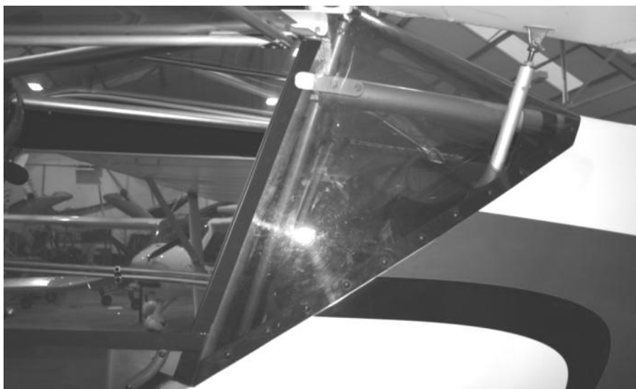
Figure 296 finished installed rear window
