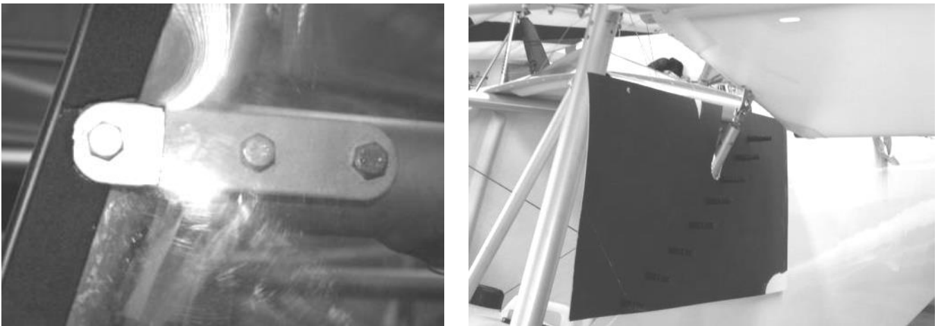
Figure 295 lexan cut around end of TU2 and template to get exact hole shape
