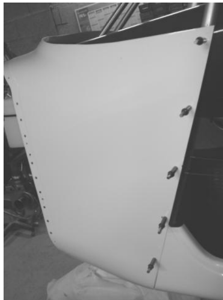
Figure 194 fixing the rear of the scuttle
