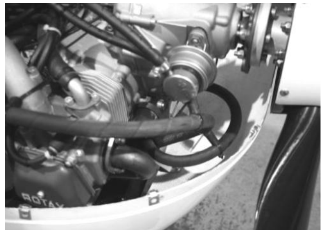
Figure 205 routing of oil hose from oil cooler connection to outlet on oil tank. Note use of cableties through short lengths of fuel tubing to act as standoffs on fuel pump and inlet manifold to secure hose.
