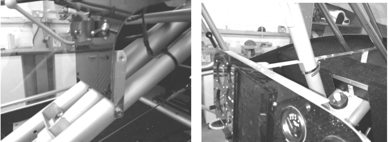
Figure 238 Instrument panel lower fixing, and instrument panel upper fixing (note - pics are of a Swift2 so firewall detail different)
