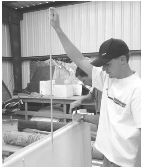
Figure 161 inserting a batten. Use your other hand to prevent the batten twisting.
