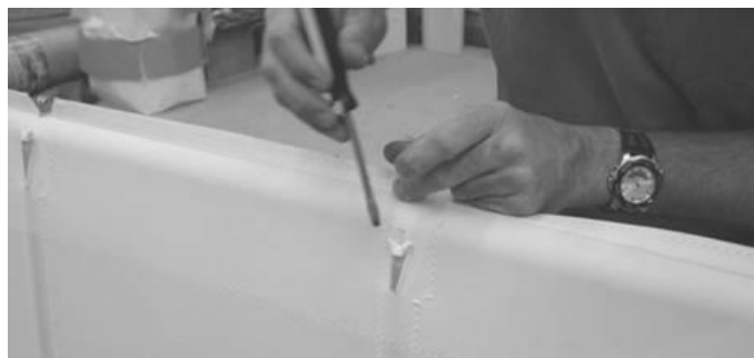
Figure 166 secure the battens in position.
