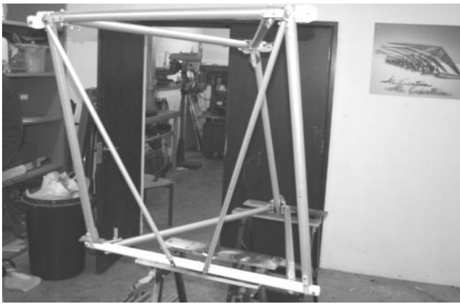
Cabin diagonals TU27 attached
