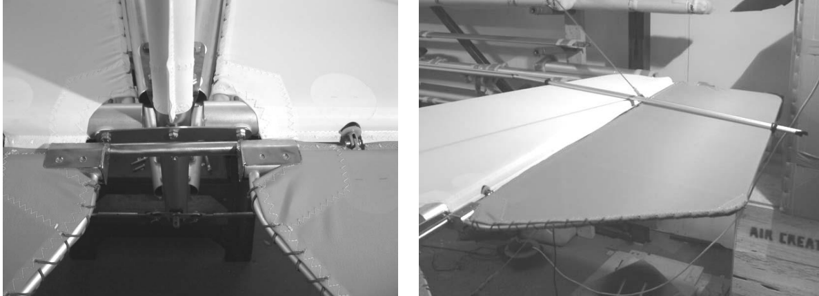
Figure 98 elevator joiner and alignment (note: Skyranger joiner shown – Nynja version has integral elevator horn).
