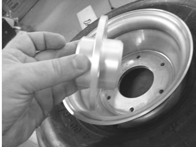
Figure 76 placing a hub against the wheel halves.
