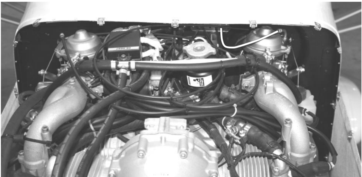
Figure 271 route of choke cable to port carburettor (in white)
