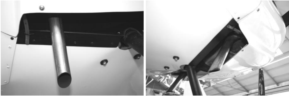
Figure 195 fixing lower edge of firewall to floor pan
