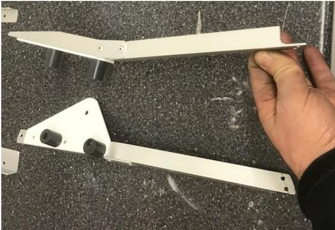
Fig 246 Finished support angle pairs.
