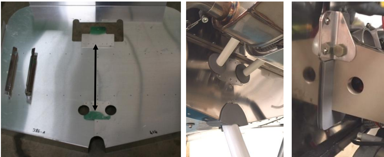
Figure 188 left - firewall closure panels – dont forget them! right - sealing
