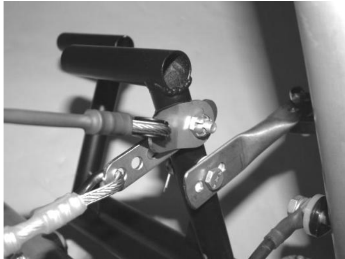
Figure 112 rudder stop cable tang fitted over rudder cable tang.
