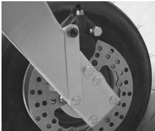
Figure 88 brake calliper mounting. Note bolts are usually the other way round, heads towards the wheel which keeps the threads away from the axle flange.
