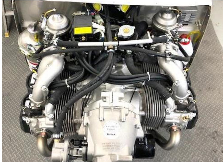
Figure 231 fuel pipe routing in engine compartment.
