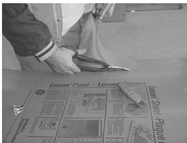
Figure 302 cutting the Lexan to the pattern.
