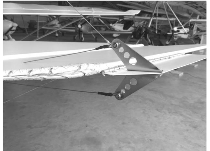
Figure 96 trim tab horns, aligned with cable bracket and hinge pin.
