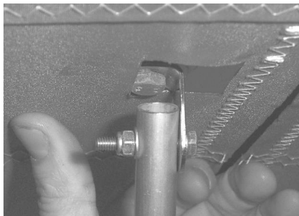
Figure 149 jury strut bracket orientation, note the adjacent seam.
