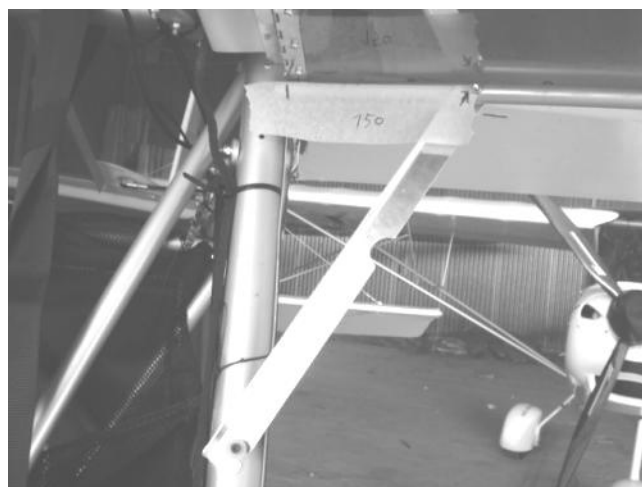
Figure 315 door open keeper, and example of an alternative fabricated stay.
