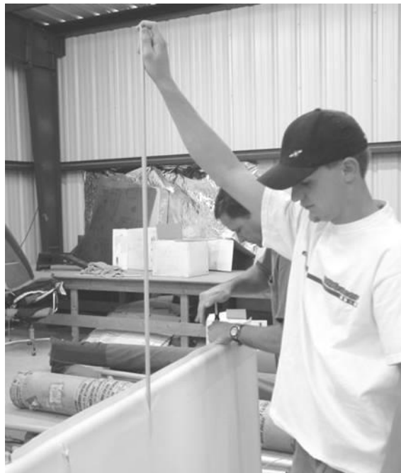
Figure 180 inserting a batten. Use your other hand to prevent the batten twisting.
