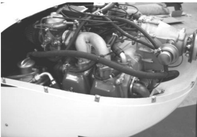
Figure 219 routing of oil hose from oil cooler connection to outlet on oil tank. Note use of cableties through short lengths of fuel tubing to act as standoffs on fuel pump and inlet manifold to secure hose.
