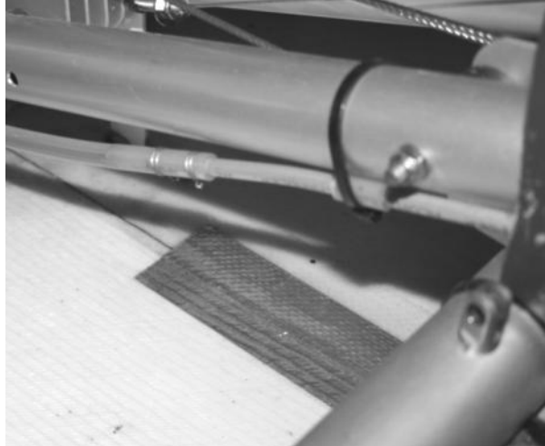
Figure 232 aluminium fuel line, cable tie and standoff.
