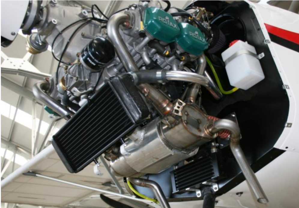
Figure 212 – exhaust in position and with heater jacket
