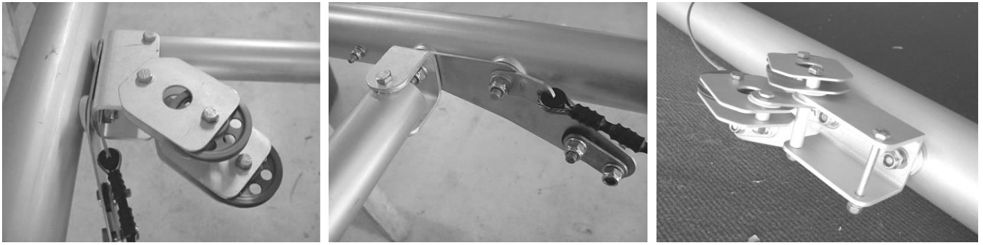
Figure 153 lift strut attachments and UKMOD aileron pulleys..
