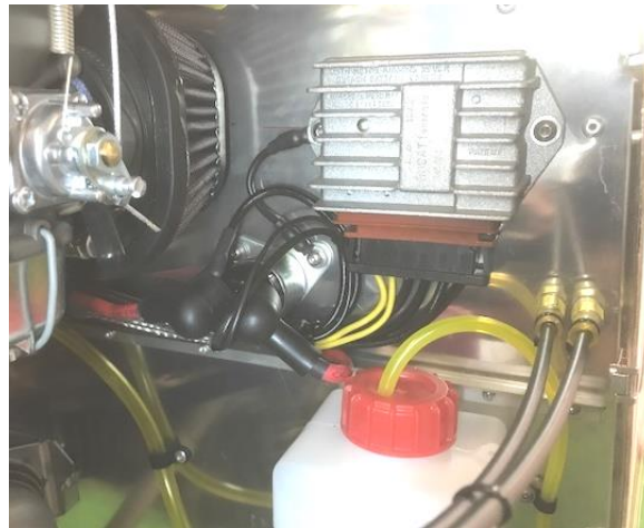
Figure 300 912 solenoid and regulator
