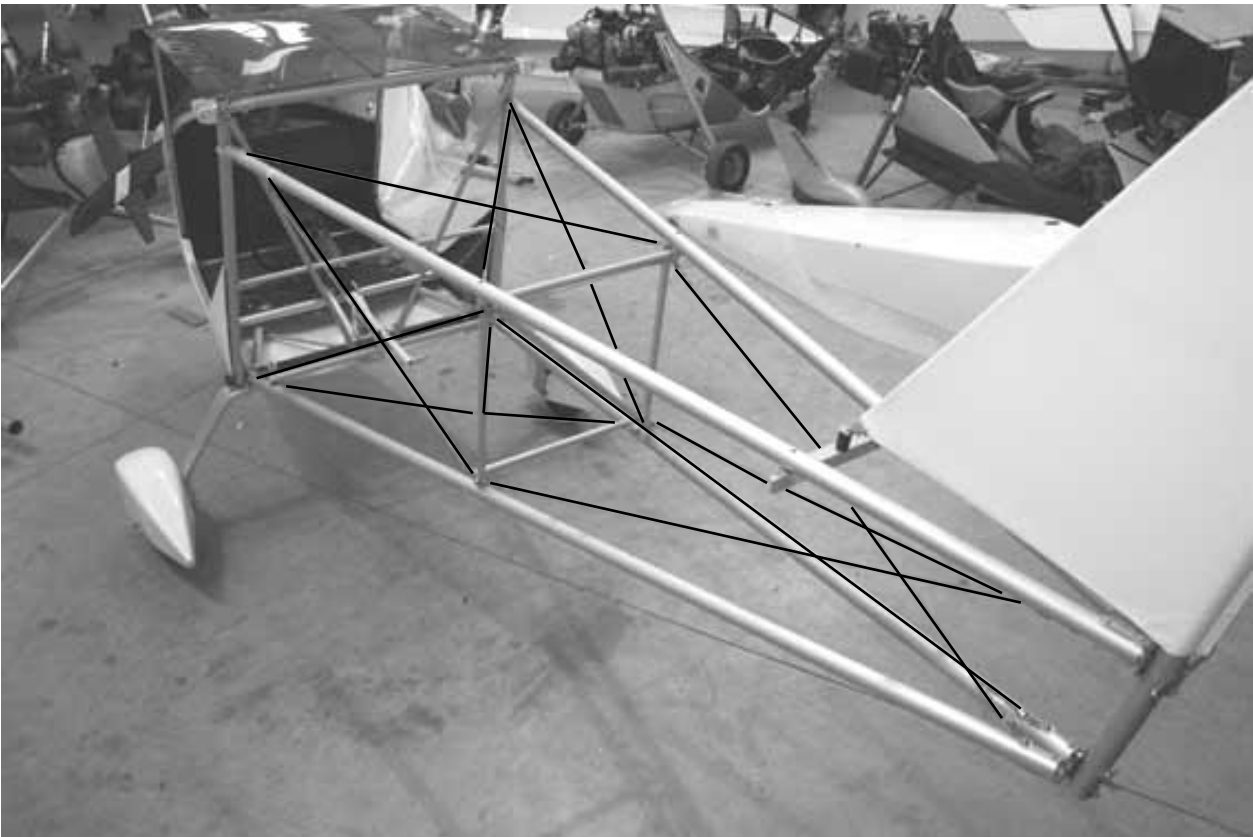
Figures 67 cable arrangement further overview (note Nynja frame shown, but same general arrangement with Swift)
