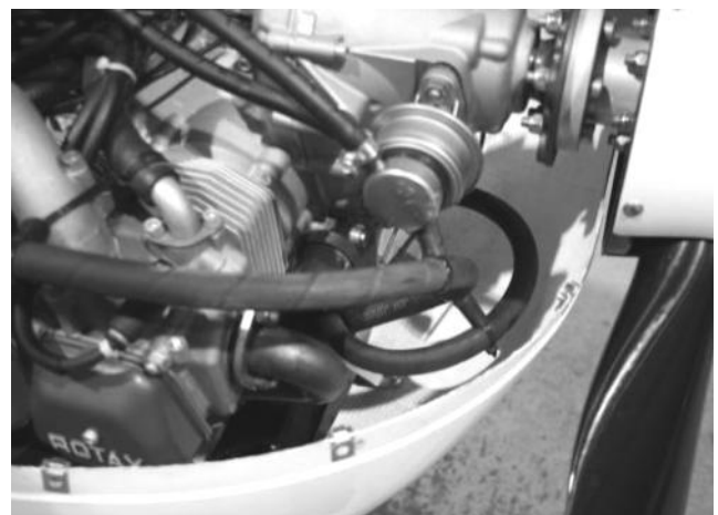
Figure 219 routing of oil hose from oil cooler connection to outlet on oil tank. Note use of cableties through short lengths of fuel tubing to act as standoffs on fuel pump and inlet manifold to secure hose.
