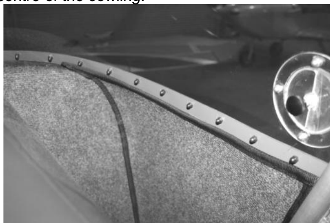
Figure 304 windscreen over lap inside cowling (note we painted the overlap to match interior fabric trimming – simply painting the composite behind black produces a nice appearance.
