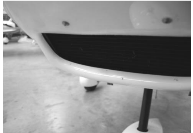
Figure 218 radiator position and attachment
