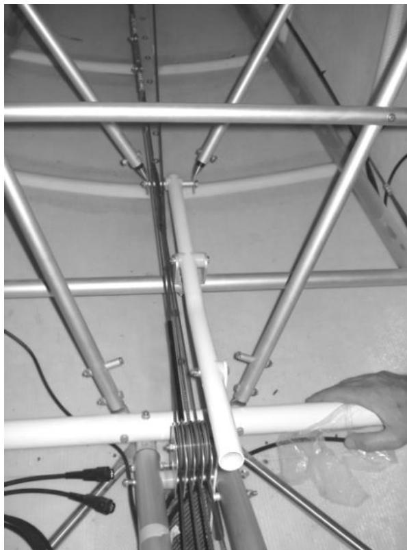
Figure 111 cable routing past flap handle.
