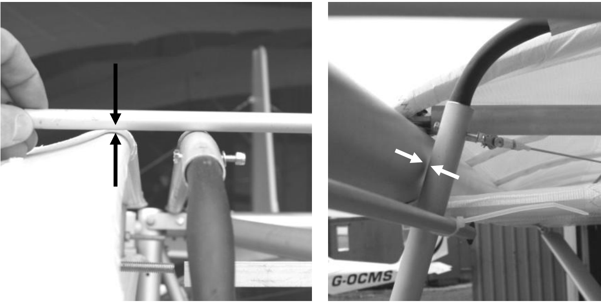
Figure 186 left – Check cabin roof tubes align with wing – level or slightly above. Right – check there is a gap of around 3-5mm here.
