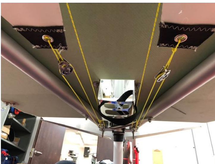
Figs 122 Lower fuselage cover and pulley arrangement
