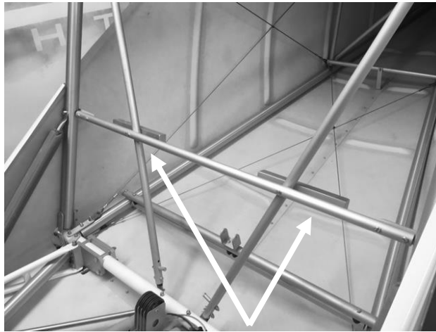
Figure 30 fuel tank wooden tank spreader pieces.
