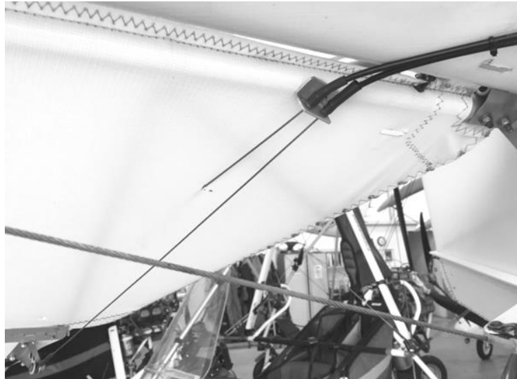
Figure 95 trimmer rear cable bracket.
