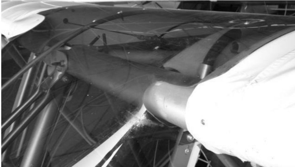
Figure 188 match up with wing so clear roof section will later fit flush like this
