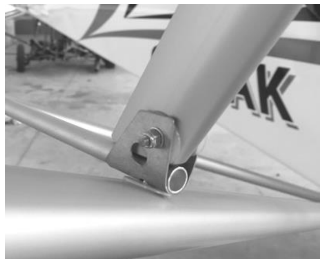
Figure 382 Rear and front lower fittings. Note orientation (looking from front)
