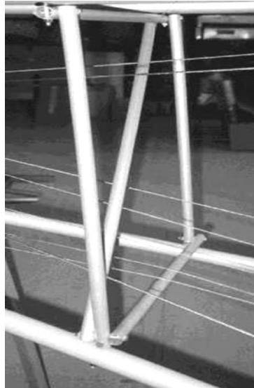
Figure 58 rear fuselage bracing frame, rear to left of photograph.
