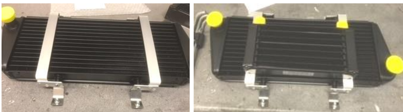
Figure 216 water radiator with brackets fitted, and with oil cooler in position.
