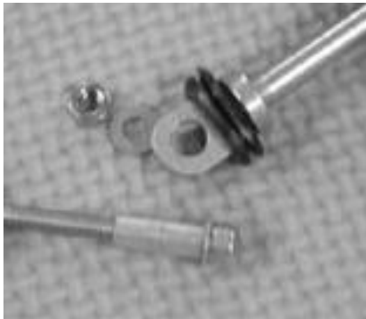
Figure 384 Upper fixing hardware. Note position of rubber grommet
