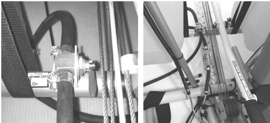
Figure 246 fuel tap, filter and connections
