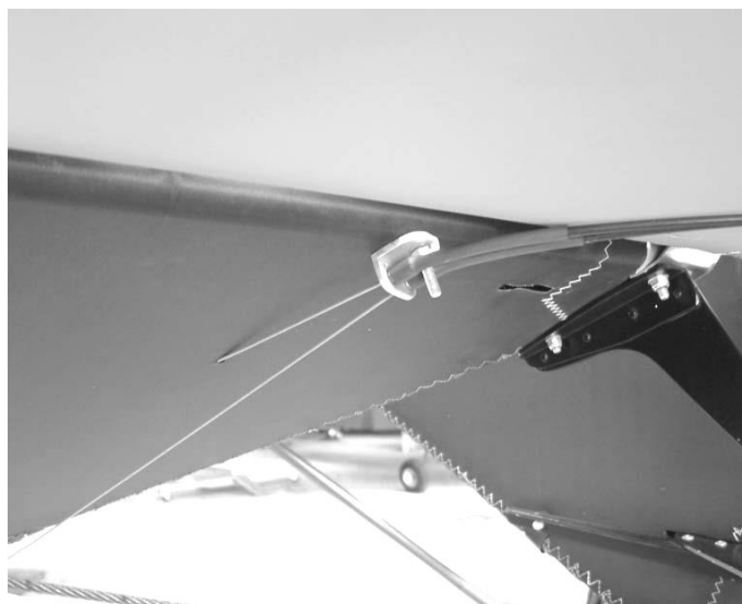
Figure 128 aft end of trimmer cables.
