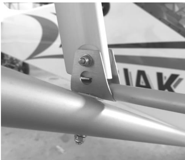
Figure 382 Rear and front lower fittings. Note orientation (looking from front)
