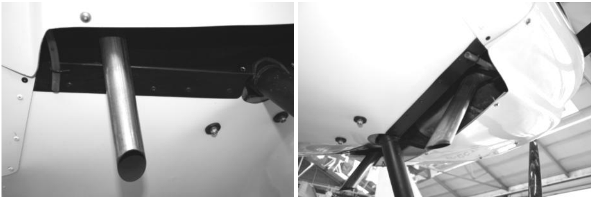
Figure 209 fixing lower edge of firewall to floor pan
