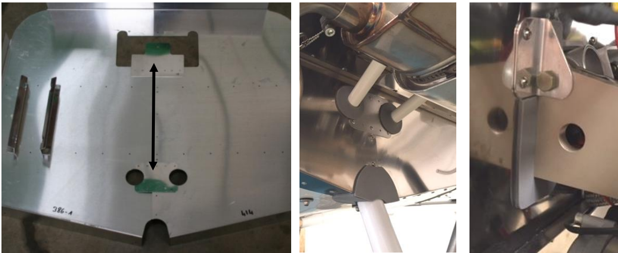
Figure 201 left - firewall closure panels – dont forget them! right - sealing
