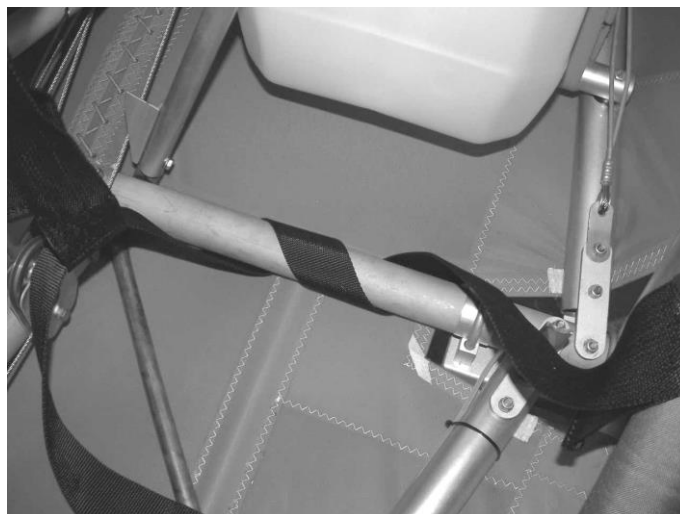
Figure 341 lap strap looped around undercarriage beam.
