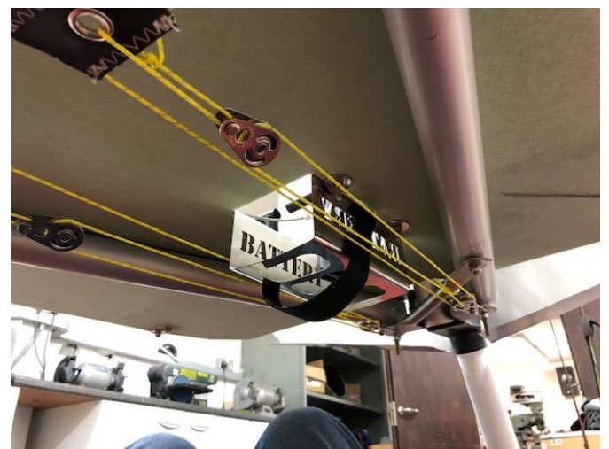
Figs 122 Lower fuselage cover and pulley arrangement
