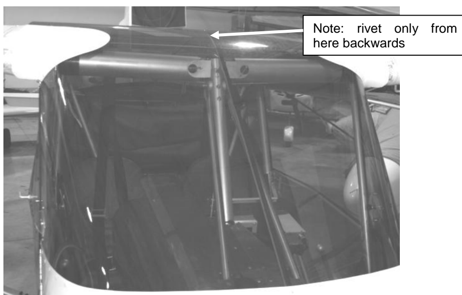
Fig 305 screen centre batten
