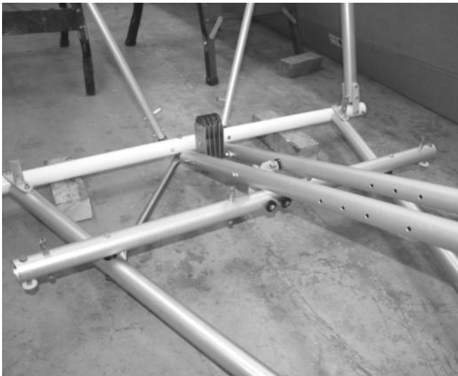
Front seat support TU15 and braces
