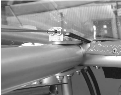
Figure 93 forward end of trimmer cables.
