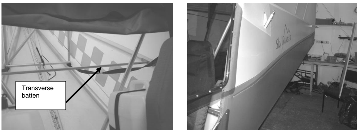
Figure 135 Transverse batten and curve produced in side of fuselage
