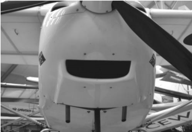
Figure 218 radiator position and attachment
