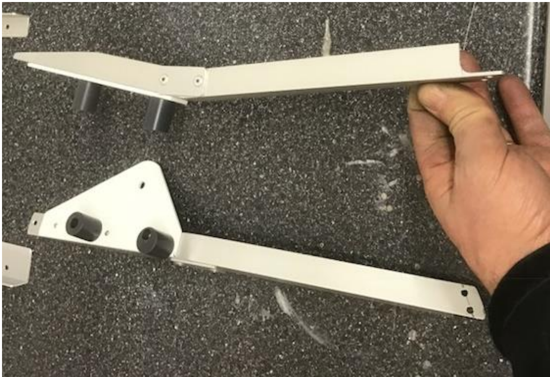
Fig 260 Finished support angle pairs.
