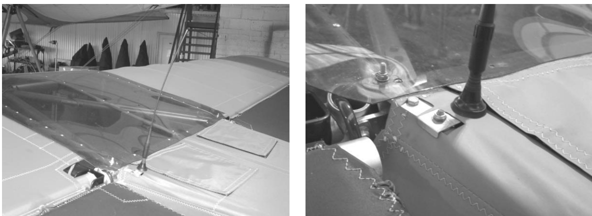
Figure 290 suggested aerial mounting.
