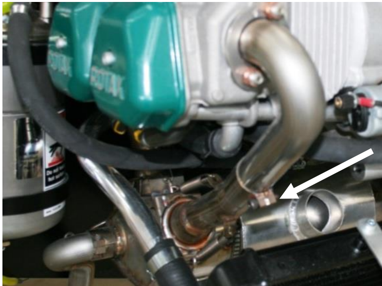
Figure 213 Port front pipe, showing clamp on sliding section
