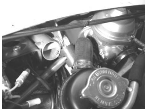
Figure 226 expansion tank and rubber elbow.
