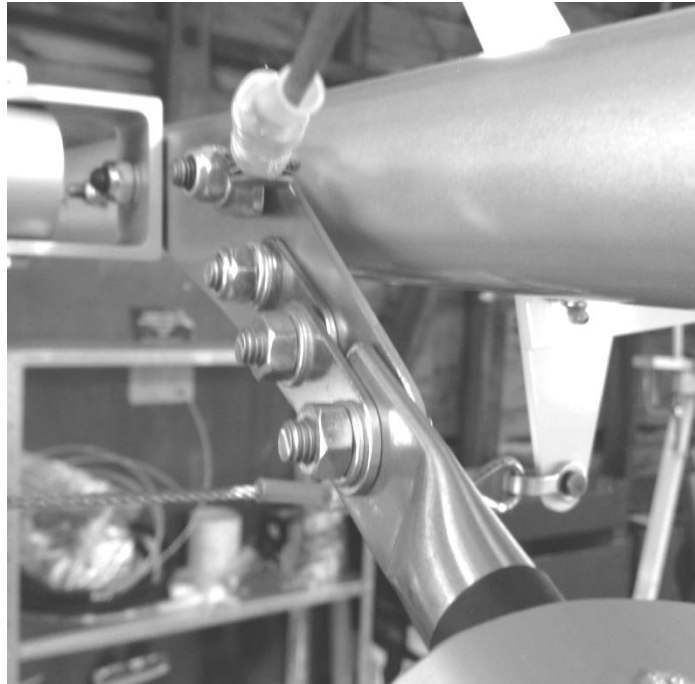
Figure 155 rear lift strut attachment (note temporary plain nuts shown – Nyloc nuts must be fitted for final assembly!).
