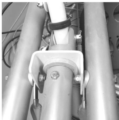
Figure 115 rudder stop cables attached to rear stick pivot.
