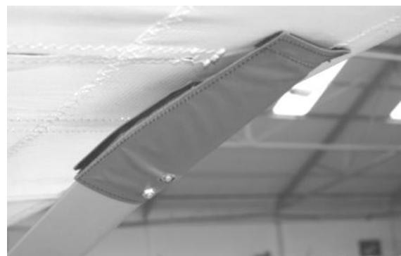
Figure 374 strut end fairings
