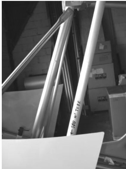
Figure 200 scuttle positioning – dont trim overlap yet, and clamp in position with upper edge around 500mm from top of door pillar tube (TU34 (note – some sanding of top edge of scuttle may be necessary to acheive a symettrical measurement – and may not be exactly 500mm)).
