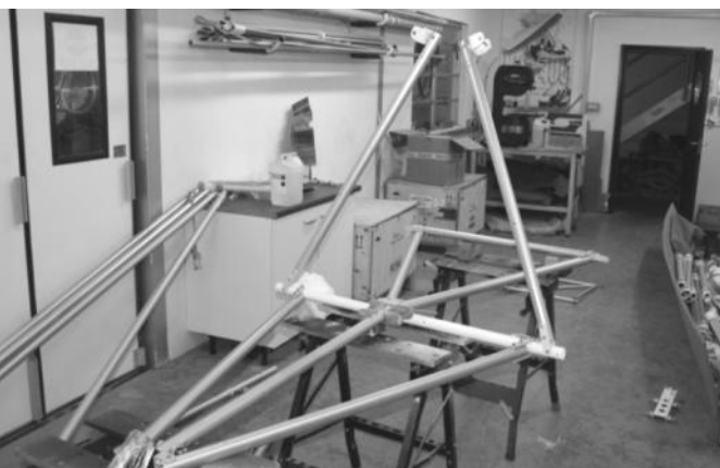
Attaching rear cabin uprights TU6
