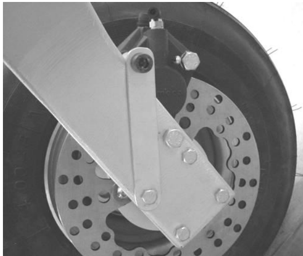
Figure 89 brake calliper mounting. Note bolts are usually the other way round, heads towards the wheel which keeps the threads away from the axle flange.
