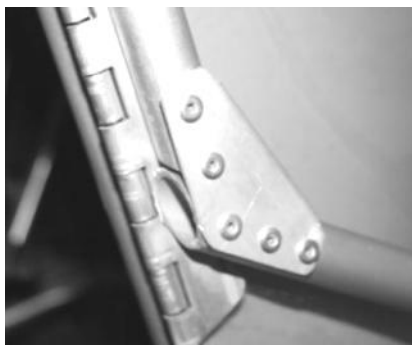
Figure 320 front end of lower door tube – shown with door open.
