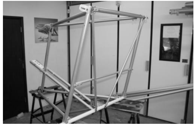
Twin TU19 tubes in position
