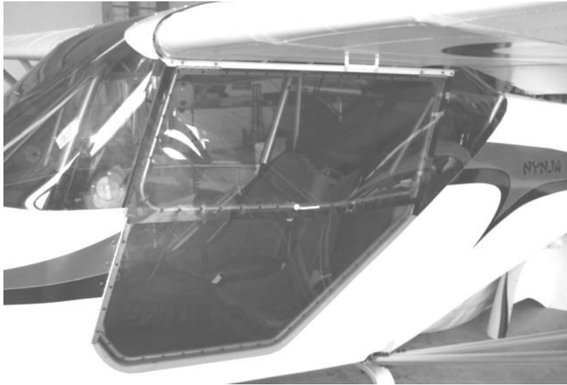
Figure 316 two piece door overview
