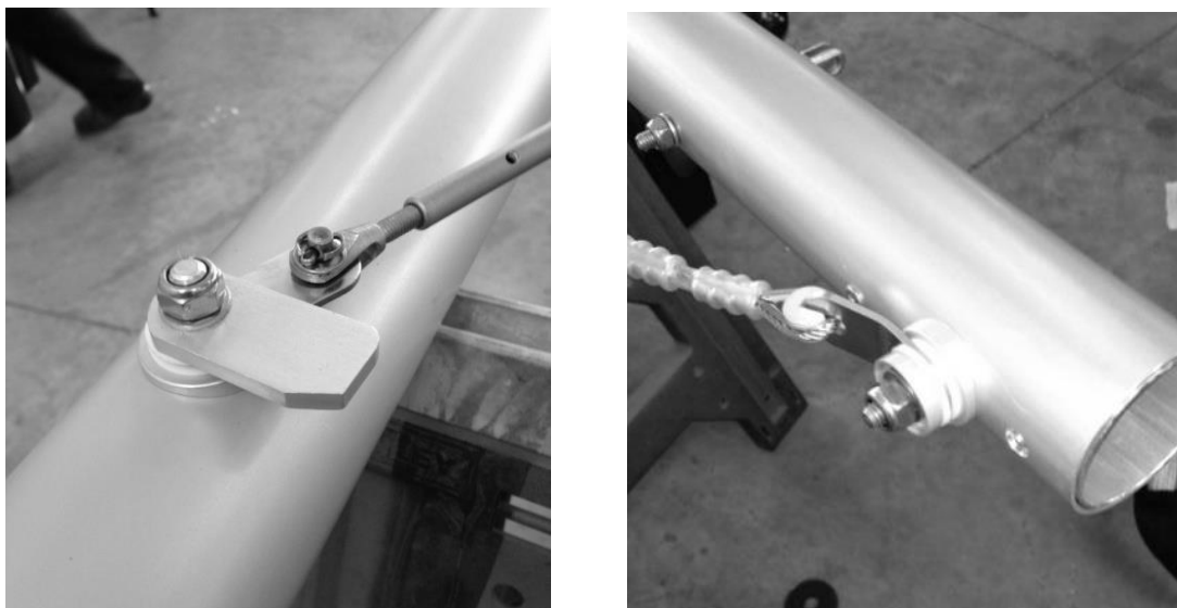
Figure 157 tensioning tube fittings, front in left photo
