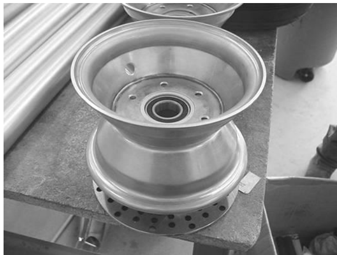
Figure 79 a wheel minus the tyre.
