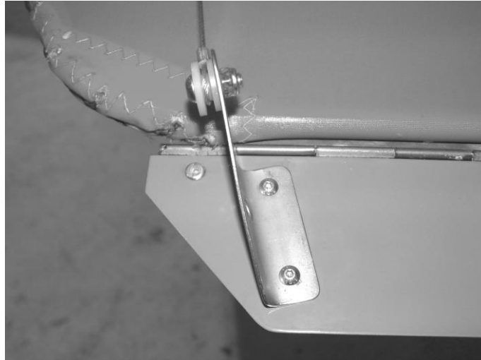
Figure 131 cable attachment on trim tab horn.
