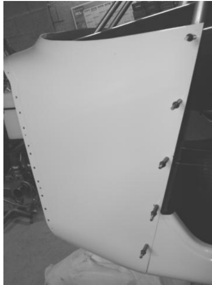
Figure 208 fixing the rear of the scuttle
