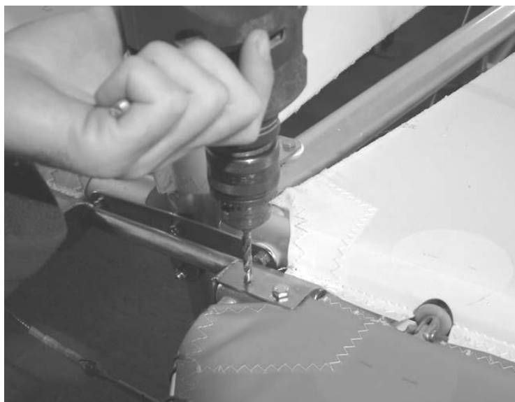
Figure 101 drilling the elevator halves.
