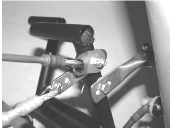
Figure 114 rudder stop cable tang fitted over rudder cable tang.
